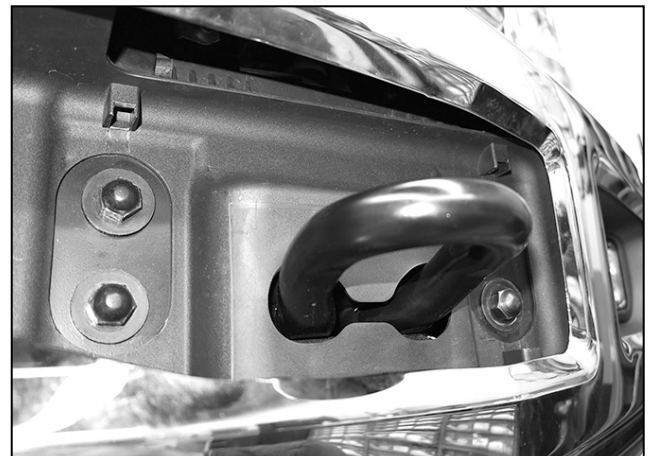
(Fig 4) Remove bumper bolts (driver side pictured)
